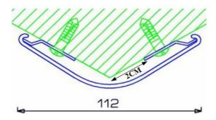
In case of failing to mount proceed to expand the angle of Zikonyl®, you have to apply pressure in the center of the profile in order to expand it's angle, ie the profile will be more open, and so will be easier to mount.
